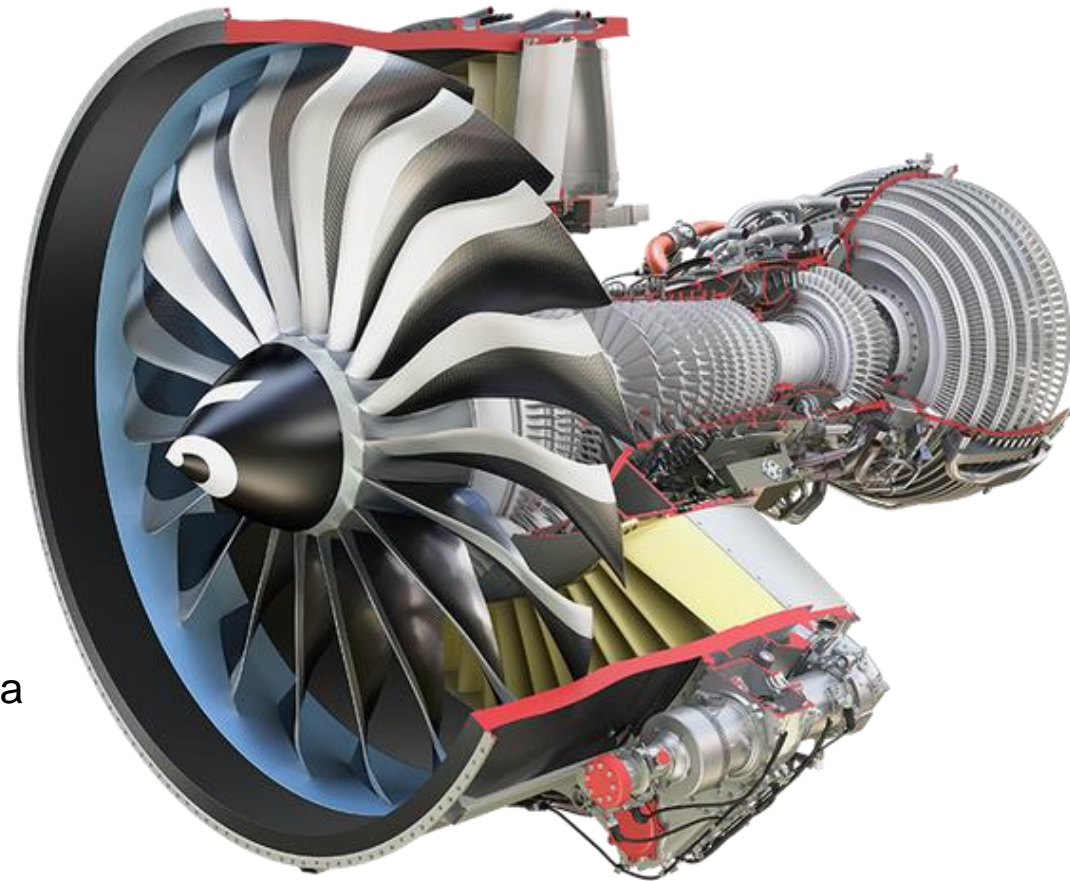
Fig.1: Modern turbofan engine - CFM International LEAP-1C [1]
